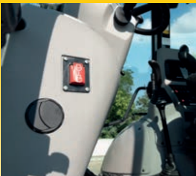
Secondary engine shut down switch
