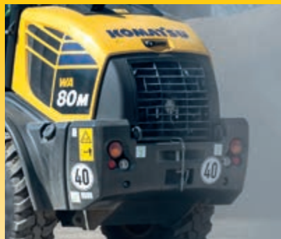
Wide core radiator with (optional) reversible fan
