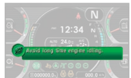
Eco guidance supports energy saving in real time (e.g. avoid long time engine idling)
