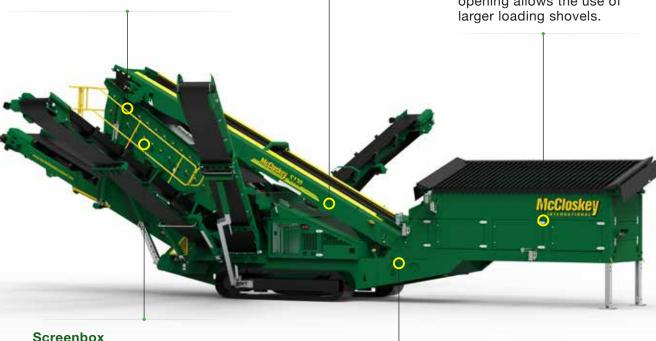
High Energy 14x5 (4200x1524mm) screenbox provides comparable product capacity with other larger class competitor's models.
