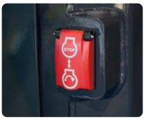
Secondary engine shutdown switch
