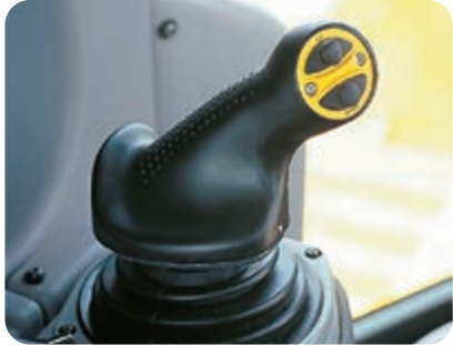
Palm Command Control System (PCCS)
