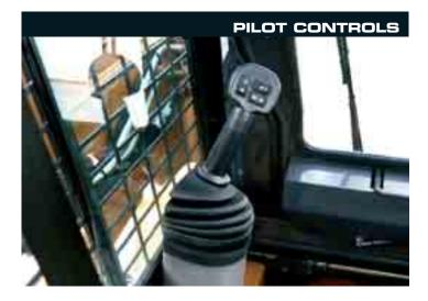
Hydraulic pilot control levers offer precision, low effort control of the machine. Straight line forward and reverse operations easier to control, increasing productivity in fine grading and dozing operations. Ease of operation boosts productivity and efficiency. Standard ISO pattern controls means direction (forward/reverse/ counter-rotation) is controlled by the left hand, and equipment (arm and bucket) controlled by the right hand.
