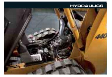
With standard auxiliary hydraulics, providing up to 83 litres/min of flow, the 440CT is well equipped to drive a wide variety of attachments. Optional High Flow hydraulics can be specified, providing up to 123 litres/min of flow for planers, stump grinders and other high flow attachments. As the 440CT can share all attachments with the popular Case skid steer range, it offers a highly versatile solution in wet, muddy or sensitive ground conditions.
