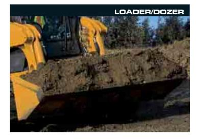
The Case 440CT has a heavy duty fully welded steel chassis and loader arms. With an operating weight of 4043 kg, the compact machine has a tipping load capacity of 2721 kg and an operating load of 1361 kg. Breakout force at the bucket is a powerful 27610 N. Case skid steers are renowned for their durable build quality and high productivity. The 440CT takes that performance to a new level, boosting productivity for the customer.
