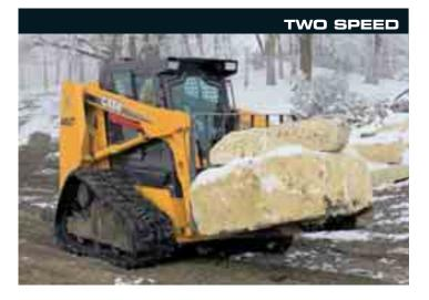
The 440CT has standard two-speed tracking, offering a maximum travel speed of 12 km/h. The final drive motors are elevated to keep them away from damaging rocks, and they use oversize bearings mounted in line with the drive sprocket for reliability and durability.
