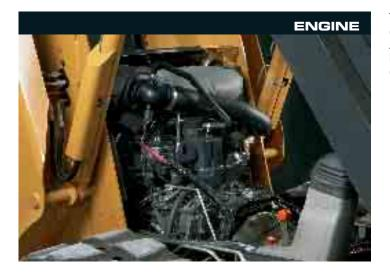
The 440CT is powered by a Case 445T/M2 turbocharged diesel engine, providing a powerful 89 hp (66 kW) at just 2300 rpm. A strong 357 Nm of torque offers more than enough rimpull to keep the machine moving in the toughest of conditions, aiding digging and loading performance.
