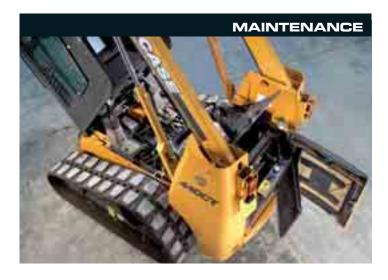
Regular service items can be easily accessed through a lift up panel on top of the engine cover and a full swing-out door to the rear of the machine. For more in-depth maintenance the entire cab structure can easily be tilted back, to provide unparalleled access to the centre of the machine.
